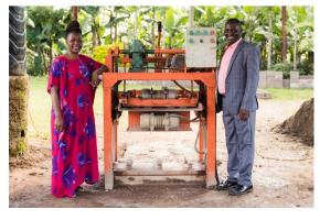
For the first time we are also professionally equipped and staffed for the brick production. After purchasing and putting into operation the new brick machine (produces four bricks at a time) production is going a lot faster. Good business is already being made, especially since customers appreciate the high-quality bricks coming from the machine. What we need to do now is optimize the processes, use the machine's full
